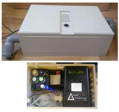
Figure 1. EB-700 platform with Alphasense sensors for gases and Dylos 1700 for \text{PM}_{10} and \text{PM}_{2.5}
