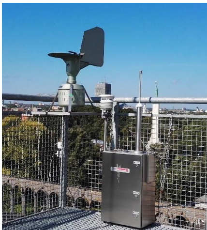
Figure 1. Burkard volumetric pollen – spore trap and GRIMM station at the monitoring site
